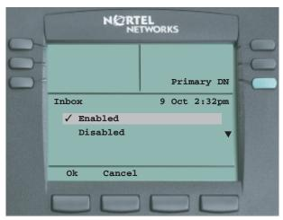
3. Press **Ok** to enable the Inbox feature that logs your calls to an inbox or press **Cancel** to return to the Assign menu (the "✓" shows that this option is selected).
